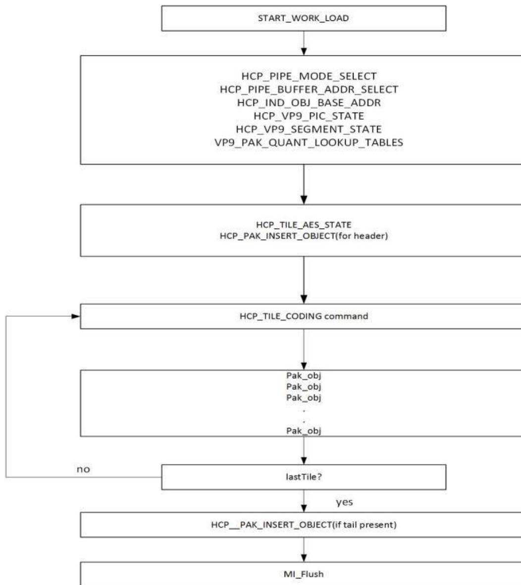
**VP9 encode command sequence for Single Pipe mode**
