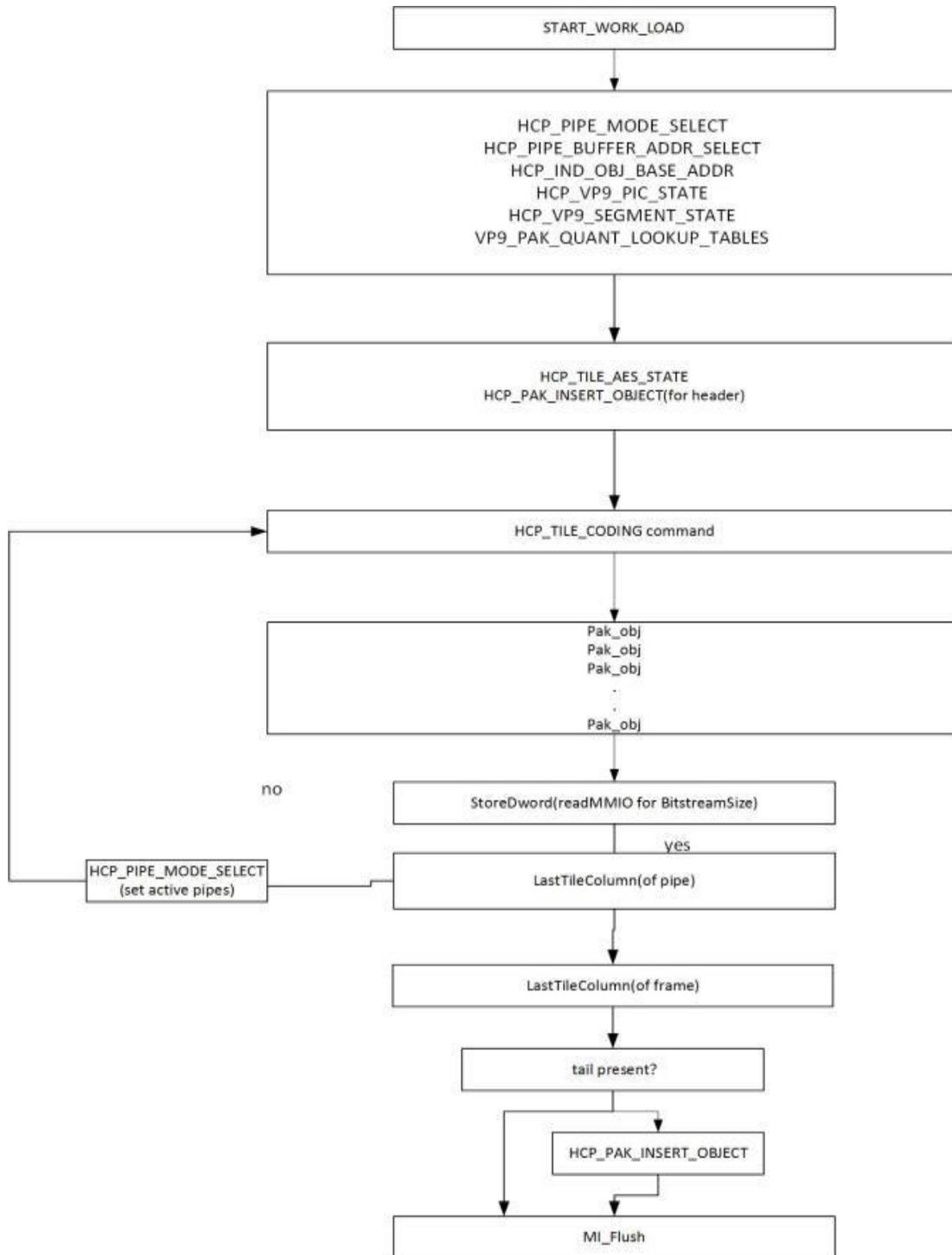
**VP9 encode command sequence in Multiple Pipes mode**
