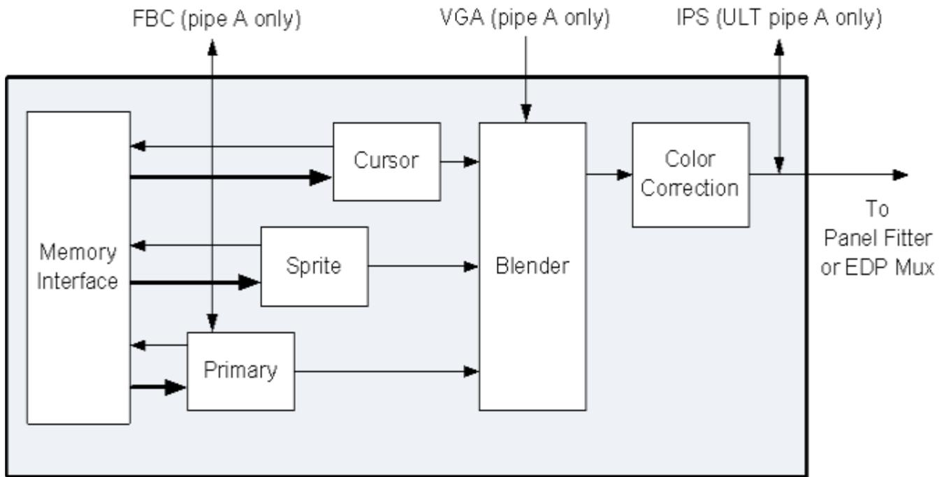
The display pipes contain the planes, blending, pipe CSC, pipe gamma, and pipe color gamut enhancement.
