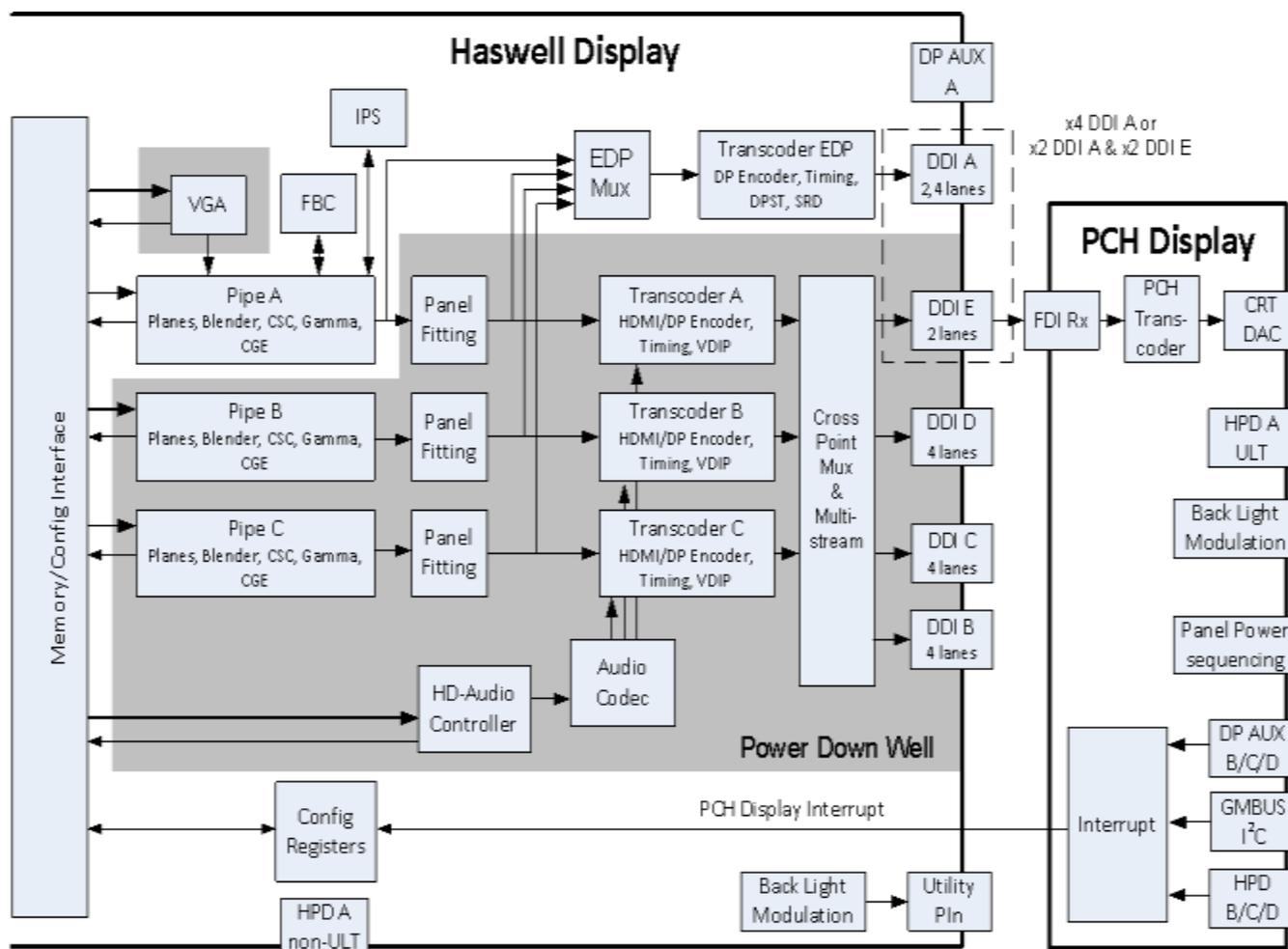
The front end of the display contains the pipes. There are three instances which are referred to as Pipe A, Pipe B, and Pipe C.
