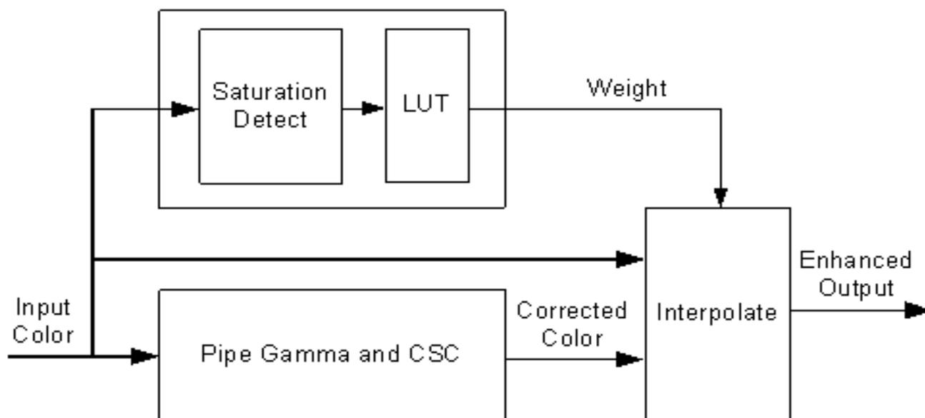
The saturation level of the pipe gamma and CSC input color is detected and used to index into a look up table (LUT) containing programmable weights. The saturation values are linearly distributed across the LUT indexes from the lowest index for lowest saturation to the highest index for highest saturation.
