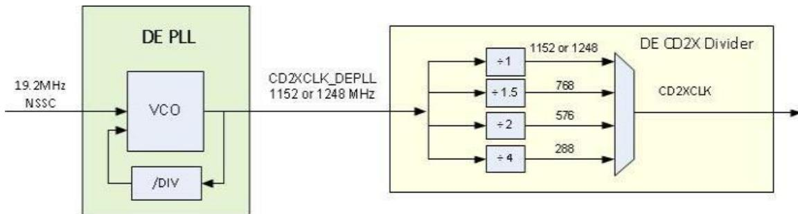
The DE PLL outputs the CD2X DE PLL clock which is the source for CD clock.
