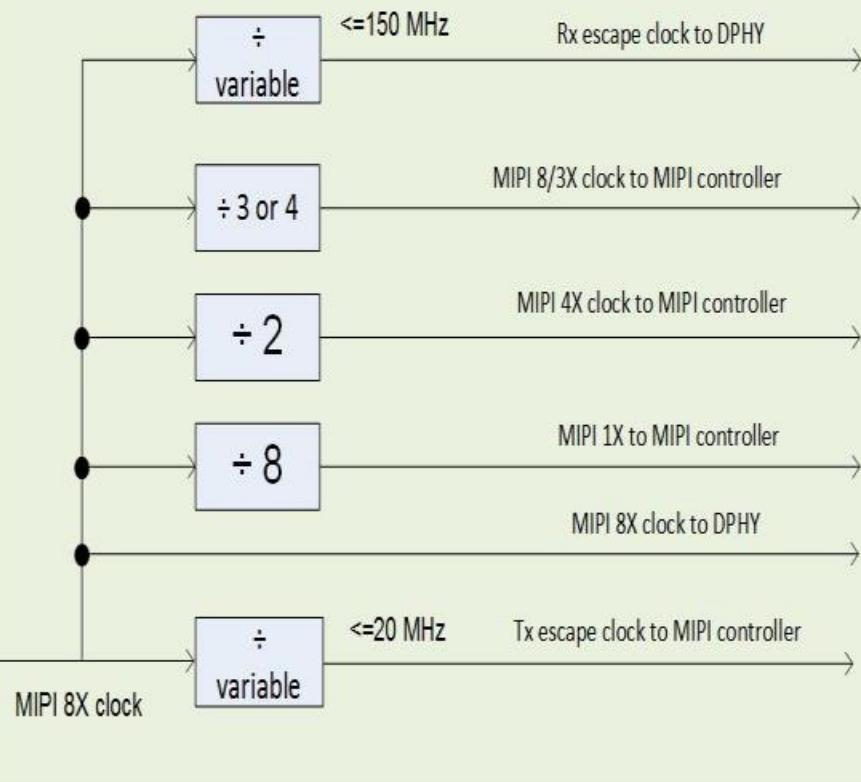
The additional MIPI clock dividers further divide the MIPI PLL 8X clock to create the different clocks for the controller and I/O PHY. The dividers are programmed through the MIPI\_CLOCK\_CTL register and must follow the restrictions there.
