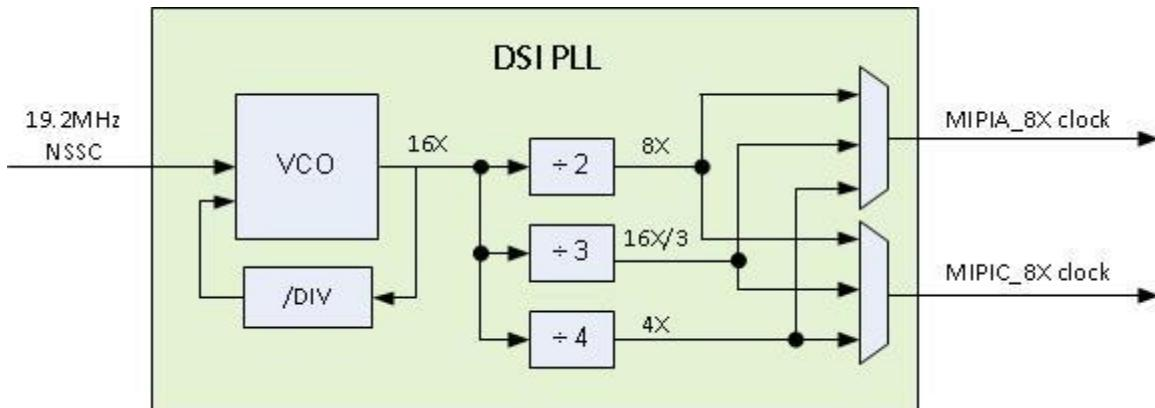
The MIPI DSI PLL block outputs the MIPI A 8X clock and MIPI C 8X clock.
