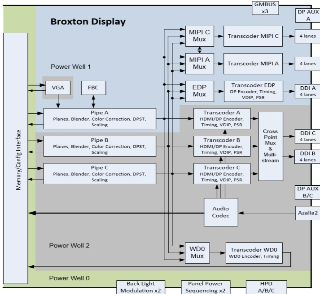
The front end of the display contains the pipes. There are three instances which are referred to as Pipe A, Pipe B, and Pipe C.
