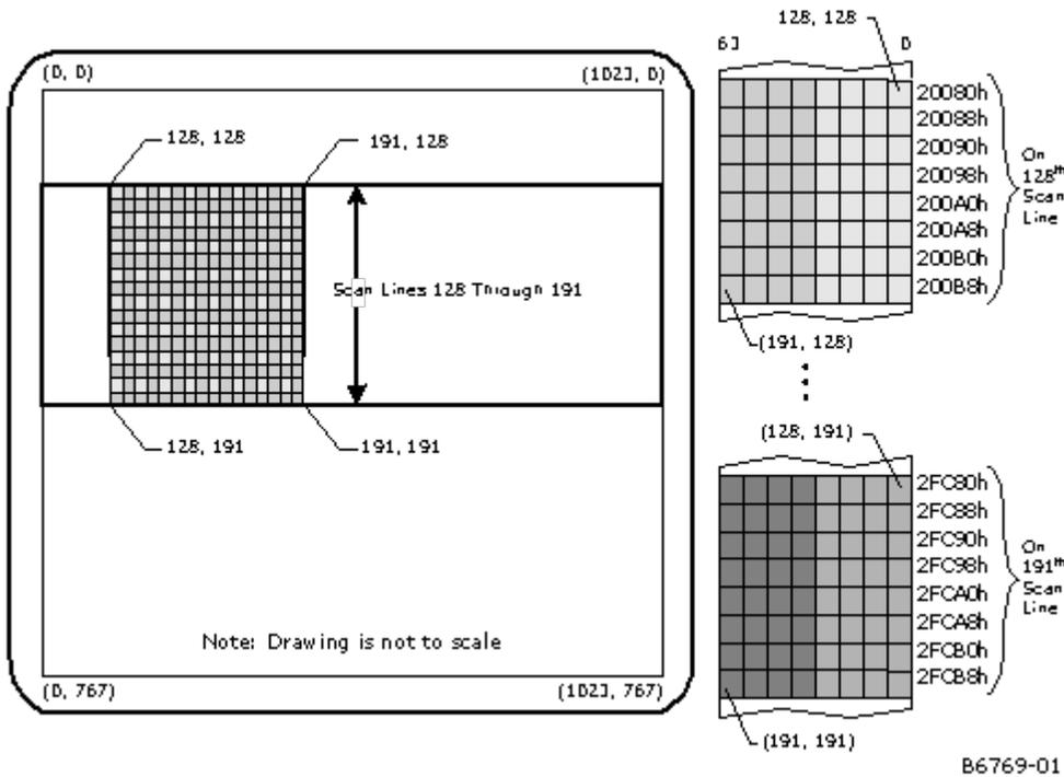
The figure above shows the end result of performing this BLT operation. The 8x8 pattern has been repeatedly copied ("tiled") into the entire 64x64 area at the destination.
