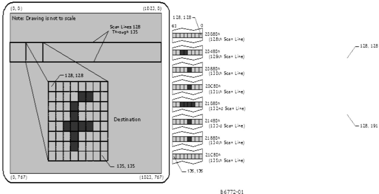
The preceding shows the end result of performing this BLT operation. Only the pixels that form part of the actual letter "f" have been drawn into the 8x8 destination location on the display, leaving the other pixels within the destination with their original gray color.
