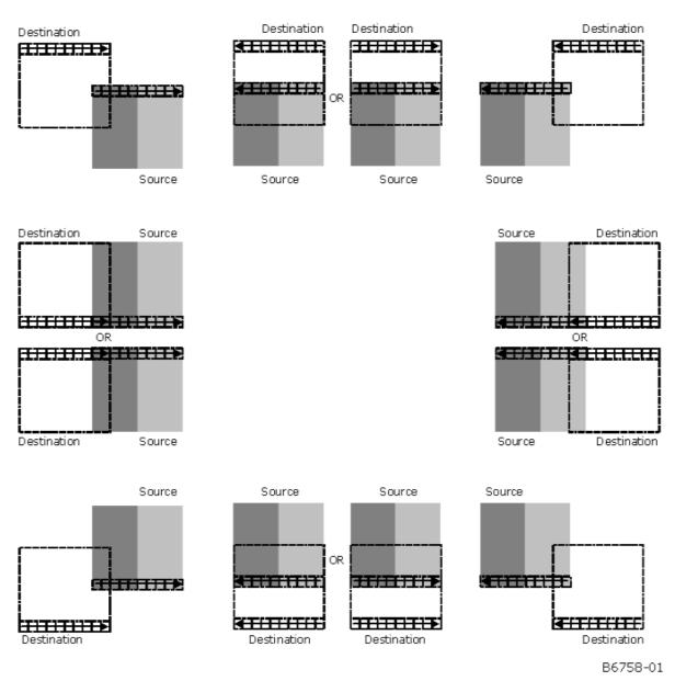
The figure above shows the recommended lines and pixels to be used as starting points in each of 8 possible ways in which the source and destination locations may overlap. In general, the starting point should be within the area in which the source and destination overlap.
