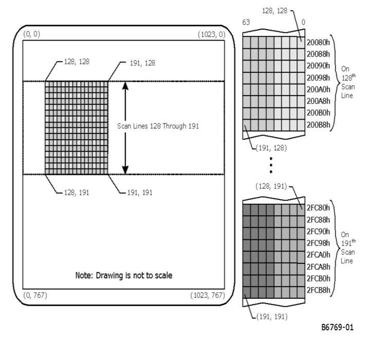
The figure above shows the end result of performing this BLT operation. The 8x8 pattern has been repeatedly copied ("tiled") into the entire 64x64 area at the destination.
