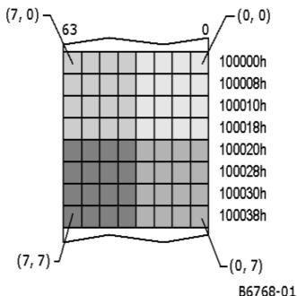
As shown in figure above, the pattern data occupies 64 bytes starting at address 100000h. As always, the pattern data represents an 8x8 array of pixels.
