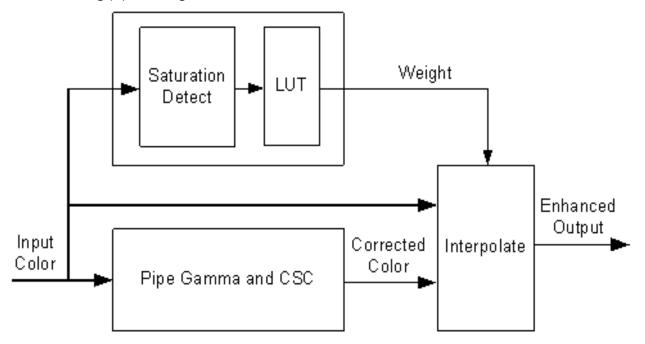
The saturation level of the pipe gamma and CSC input color is detected and used to index into a look up table (LUT) containing programmable weights. The saturation values are linearly distributed across the LUT indexes from the lowest index for lowest saturation to the highest index for highest saturation.
