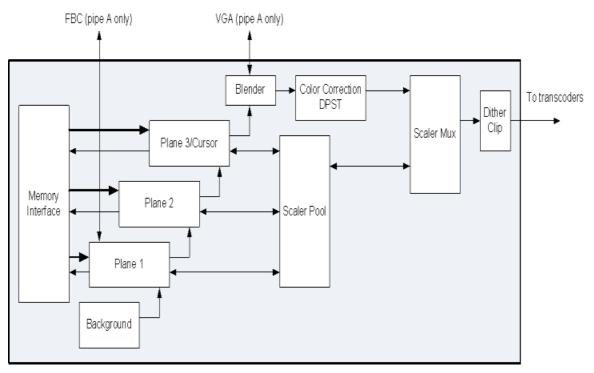
The display pipes contain the planes, blending, color correction, DPST, scaling, dithering, and clipping.
