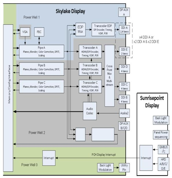
The front end of the display contains the pipes. There are three instances which are referred to as Pipe A, Pipe B, and Pipe C.
