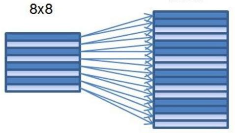
VertDownSamplingEnb is used to convert an input chroma422 to an output chroma420 in the surface format NV12. To enable this flag, the input should be interleaved Scan, InputFormatYUV should be set to YUV422H\_2Y or YUV422H\_4Y, and OutputFormatYUV should be set to NV12. Combined with AvgDownSampling flag, the following table and figures show the down-sampling methods.
