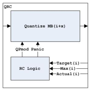
Macroblock level rate control is handled by the RC logic and the quantization logic.
