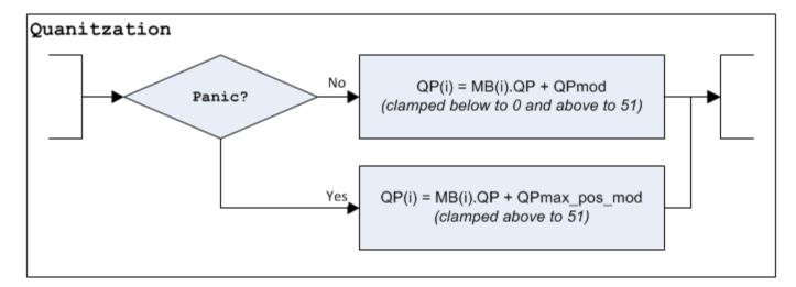
The signals QPmod and panic are generated by the RC logic based on data feedback from BSP. A flowchart of the RC logic is given below.
