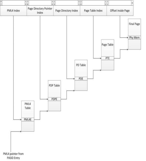
64bit (48b canonical) address requires 4-levels of page table format where the context carries a pointer to highest level page table (PML4 pointer) via PASID. The rest of the walk is normal page walk thru various levels.
