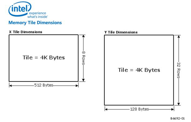
The pitch of a tiled enclosing region must be an integral number of tile widths. The 4KB tiles within a tiled region are stored sequentially in memory in row-major order.
