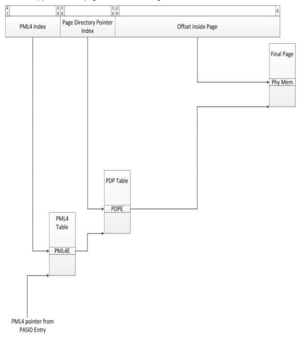
For the support for 1GB page size, the following mechanism is needed.
