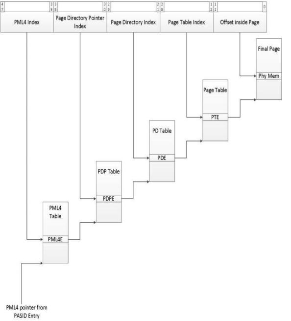
A 64 bit (48b canonical) address requires 4 levels of page table format where the context carries a pointer to highest level page table (PML4 pointer) via PASID. The rest of the walk is normal page walk thru various levels.
