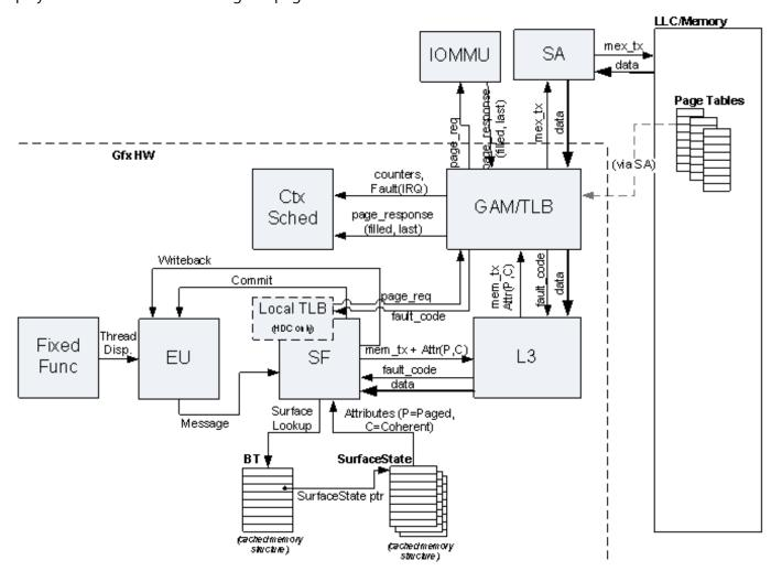
On a faultable context GAM is the interfacing HW block for Page Request and Page Response queues. Both queues are used to communicate with SW layer. For some fault modes (see "page fault modes"), the page faults need to be reported to different places. This section outlines these interfaces (excluding the page request/response interface which is tracked in a different section).
