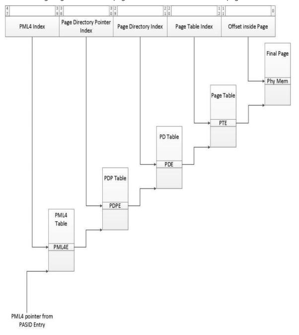
A 64-bit (48b canonical) address requires 4-levels of page table format where the context carries a pointer to the highest level page table (PML4 pointer) via PASID. The rest of the walk is a normal page walk thru the various levels.
