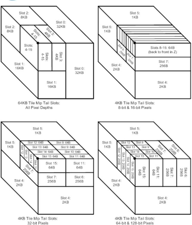
The offsets into the mip tail tile are given by the following table for each LOD in the mip tail. Note that many of the higher LODs are not possible given surface size constraints, but they are listed here for reference. The offsets given here need to be added to the LODs offset computed earlier to obtain the offset into the surface LOD<sub>L</sub>.
