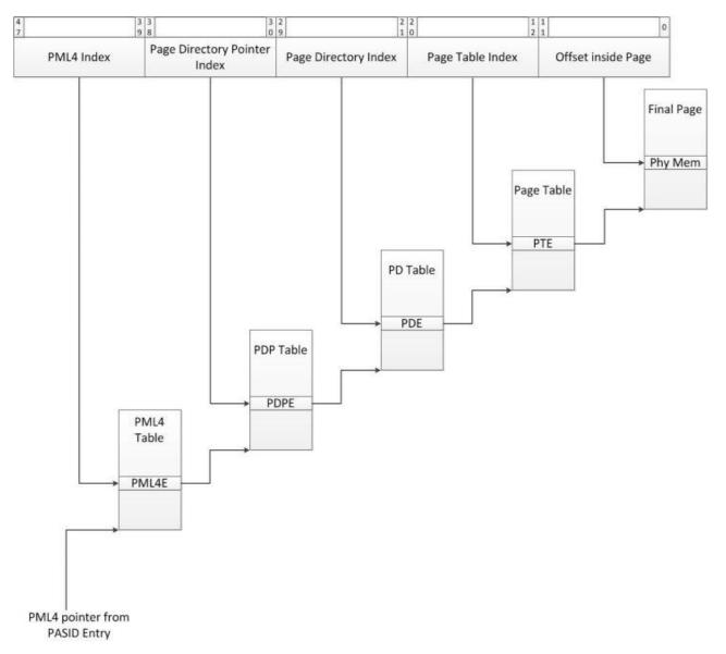
64bit (48b canonical) address requires 4-levels of page table format where the context carries a pointer to highest level page table (PML4 pointer) via PASID. The rest of the walk is normal page walk thru various levels.
