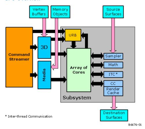
The subsystem consists of an array of *execution units* (*EUs*, sometimes referred to as an array of *cores*) along with a set of *shared functions* outside the EUs that the EUs leverage for I/O and for complex computations. Programmers access the subsystem via the 3D or Media pipelines.
