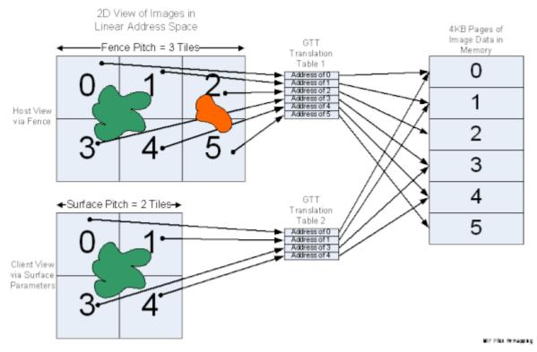
Refer to the "Graphics Translation Table (GTT) Range (GTTADR) & PTE Description" in *Memory Interface Registers* for details on PTE formats and programming information. Refer to the *Memory Data Formats* chapter for device-specific details/restrictions regarding the placement/storage of the various data objects used by the graphics device.
