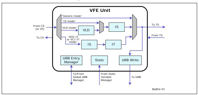
MEDIA\_STATE\_POINTERS command configures VFE in one of the three modes using. Mode switching requires media pipeline state change.
