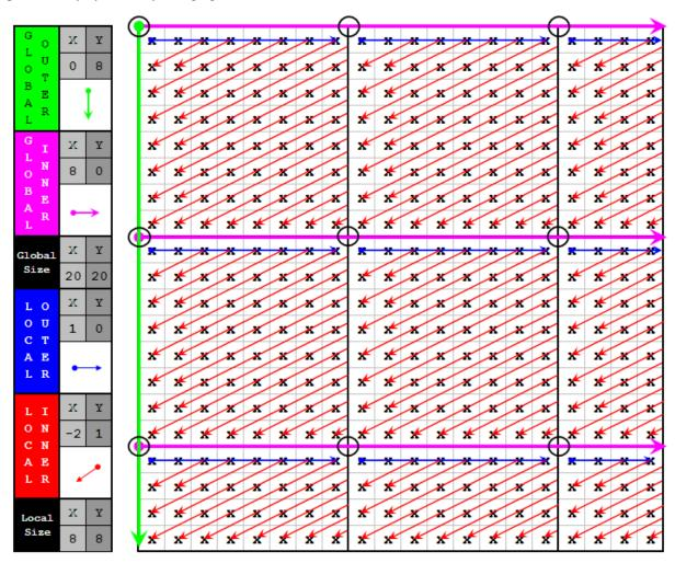
The global loop will always resolve to be the upper-left corner of the local loop, shown above black circles. Note that local loop can still start in any corner of the local block, but the local (0,0) will always be the location where global loop begins the local loop, hence the upper-left corner.
