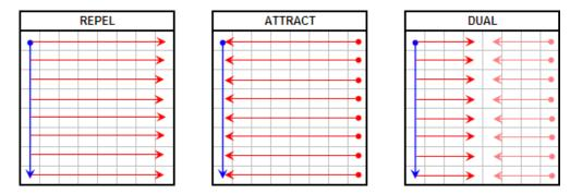
In Dual mode, the sequence will alternate between two half-walks such that every-other output would go to the same slice. This effect will produce a more balanced workload to two slices as shown in the example below where the color of the block represents which slice it was dispatched to. This is the walker's approach to fine-grained parallelism.
