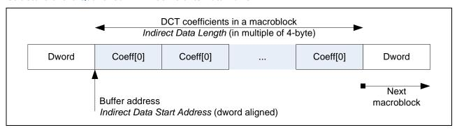
Each non-zero coefficient in the indirect data buffer is contained in a doubleword-size (32-bit) data structure containing the coefficient index, end of block (EOB) flag and the fixed-point coefficient value in 2's compliment form.
