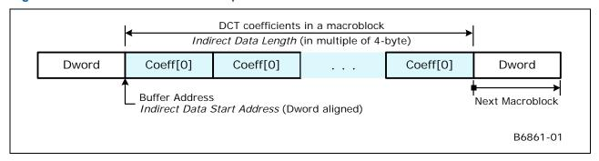
Each non-zero coefficient in the indirect data buffer is contained in a doubleword-size data structure containing the coefficient index, end of block (EOB) flag and the fixed-point coefficient value in 2's compliment form. As shown in
