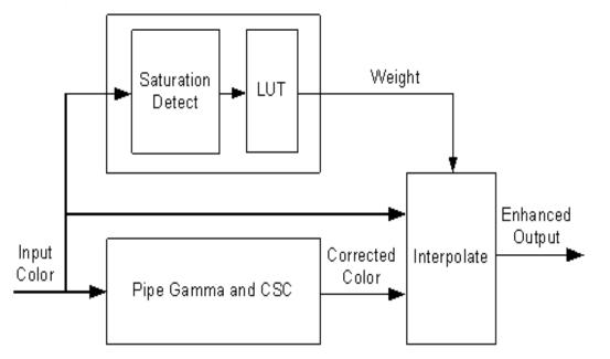
The saturation level of the pipe gamma and CSC input color is detected and used to index into a look up table (LUT) containing programmable weights. The saturation values are linearly distributed across the LUT indexes from the lowest index for lowest saturation to the highest index for highest saturation.
