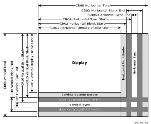
**Group 0 Protection:** In the original VGA, CR[0:7] could be made write-protected by CR11[7]. In BIOS code, this write protection is set following each mode change. Other protection groups have no current use, and would not be used going forward by the BIOS or by drivers. They are the result of an industry fad some years ago to attempt to write protect other groups of registers; however, all such schemes were chip specific. Only the write protection (Group 0 Protection) is supported.
