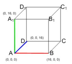
The LUT entries should start at A and end at  $C_1$  following the sequence specified below.
