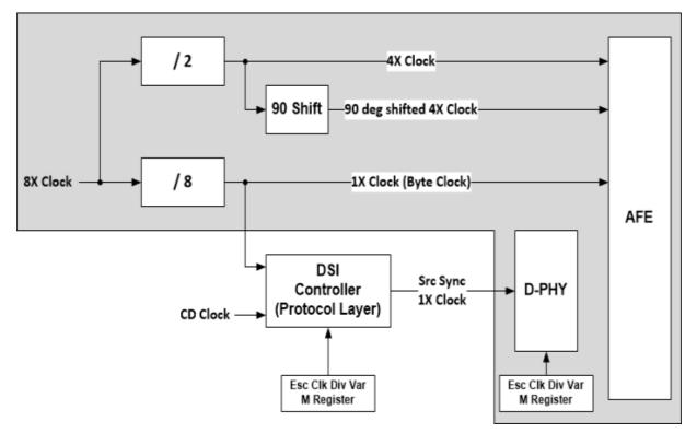
The MIPI DSI clocks are used for the DSI 0 and DSI 1 ports and transcoders.
