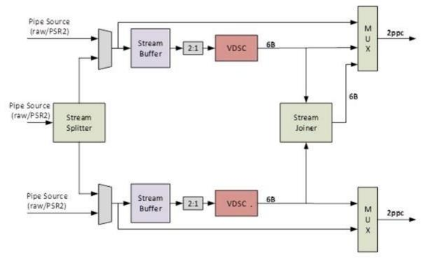
The following datapath options are supported in the VESA based compression engine. The top mux output is designated as left (front) and bottom mux output is designated as right (back) in the case of split streams. Stream joiner output can only feed into the top mux output.
