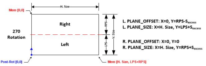
Note that Software should ensure that the horizontal Plane position for the image in the right Pipe is zero (i.e. there should be no positional offset of the image with respect to the seam)
