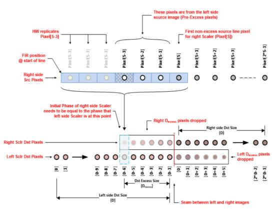
The following equation is used to determine the phase that the right-side Scaler needs to start at.
