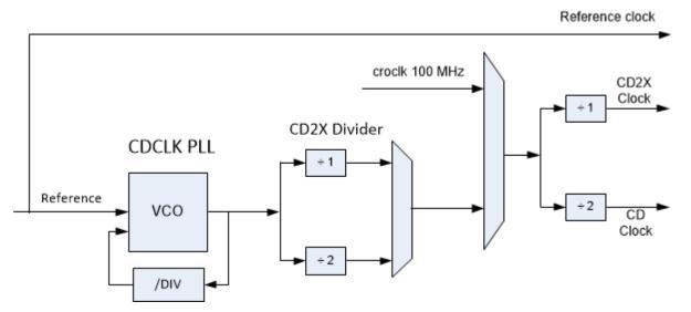
The CDCLK PLL is the main source for CD clock. A programmable divider inside the PLL controls the PLL frequency. The CD2X Divider after the PLL provides additional dividing to create the CD2X clock used by the display engine. The divider value must be set to account for the reference frequency for in the **DSSM** Reference Frequency field.
