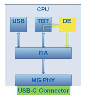
The USB type C ports are integrated into the CPU. Each type C port is shared between USB, thunderbolt (TBT), and display engine.
