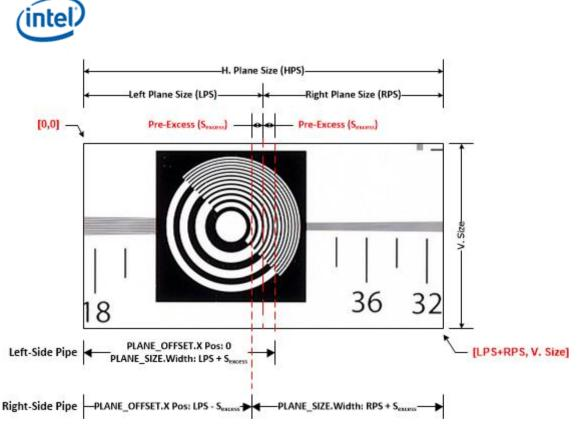
Using the figure above as a reference, to split the image in memory across the two Pipes.
