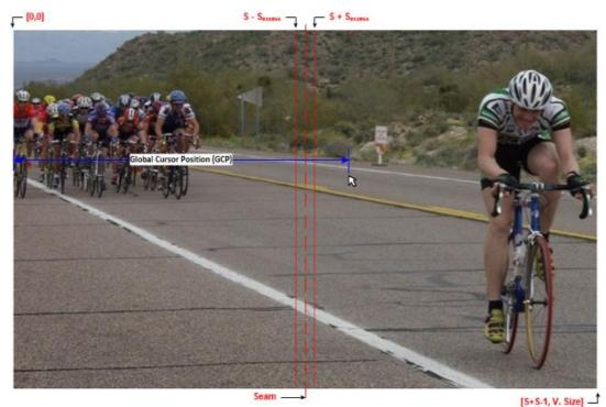
The horizontal position of the Cursor will be referred to as the global cursor position (GCP) that will span across both Pipe source windows from 0 to (2\*S)-1.
