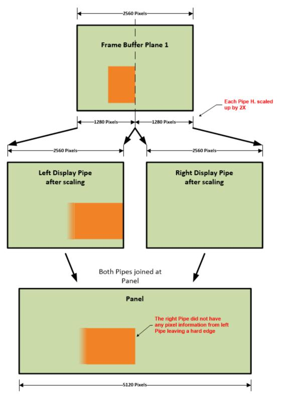
By adding some overlapping pixels of the split image around the seam, the Scalers within each Pipe will be able to correctly filter across the seam. At the end of the Pipe (before the image is delivered to the Port) the post-scaled overlap pixels will be dropped.
