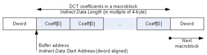
Each non-zero coefficient in the indirect data buffer is contained in a doubleword-size data structure consisting of the coefficient index, end of block (EOB) flag and the fixed-point coefficient value in 2's compliment form. As shown in Structure of a transform-domain residue unit, *index* is the row major 'raster' index of the coefficient **within a transform block** (*please note that it is not converted to 8x8 block basis*). A coefficient is a 16-bit value in 2's complement.
