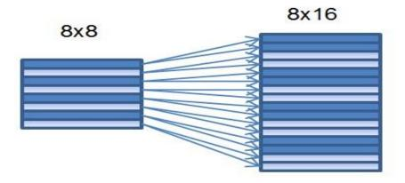
VertDownSamplingEnb is used to convert an input chroma422 to an output chroma420 in the surface format NV12. To enable this flag, the input should be interleaved Scan, InputFormatYUV should be set to YUV422H\_2Y or YUV422H\_4Y, and OutputFormatYUV should be set to NV12. Combined with AvgDownSampling flag, the following table and figures show the down-sampling methods.
