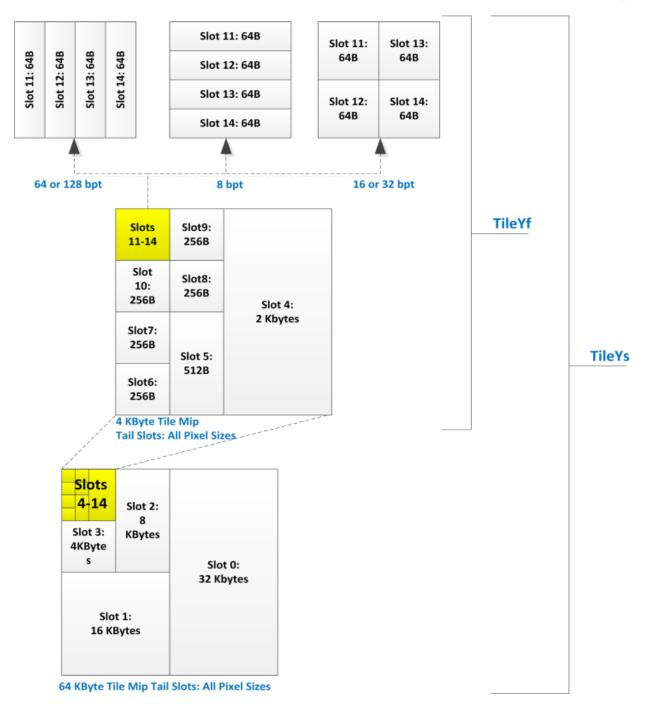
The offsets into the Mip Tail tile are given by the following table for each LOD in the Mip tail. Each entry in the table is a horizontal ( $M_U$ ) and vertical ( $M_V$ ) position (in texels) from the upper left corner of the Mip Tail. If LOD >= S (starting LOD for MIP Tail), then these Mip Tail offsets must be added to the LODU<sub>L</sub> and LODV<sub>L</sub> calculated above.
