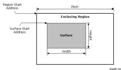
The simplest storage format is the *linear* format (see *Linear Surface Layout*), where each row of the operand is stored in sequentially increasing memory locations. If the surface width is less than the enclosing region's pitch, there will be additional memory storage between rows to accommodate the region's pitch. The pitch of the enclosing region determines the distance (in the memory address space) between vertically-adjacent operand elements (e.g., pixels, texels).
