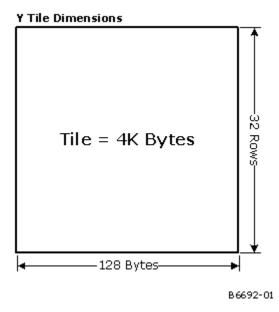
The pitch of a tiled enclosing region must be an integral number of tile widths. The 4KB tiles within a tiled region are stored sequentially in memory in row-major order.
