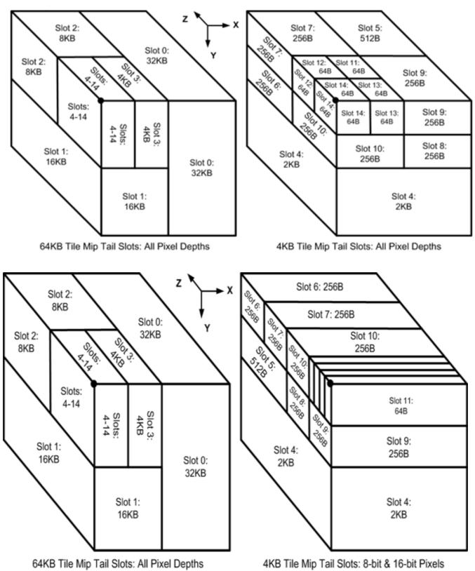
The offsets into the mip tail tile are given by the following table for each LOD in the mip tail. Note that many of the higher LODs are not possible given surface size constraints, but they are listed here for
