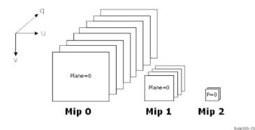
**Surface Pitch** defines the distance in bytes between rows of the surface. **Surface QPitch** specifies the distance in rows between R-slices. QPitch should allow at least enough space for any mips that may be present.
