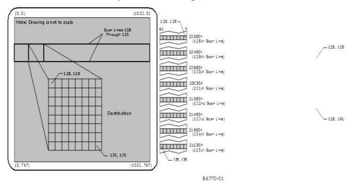
The figure above shows the display on which this letter "f" is to be drawn. As shown in this figure, the entire display has been filled with a gray color. The letter "f" is to be drawn into an 8x8 region on the display with the upper left-hand corner at the coordinates (128, 128).
