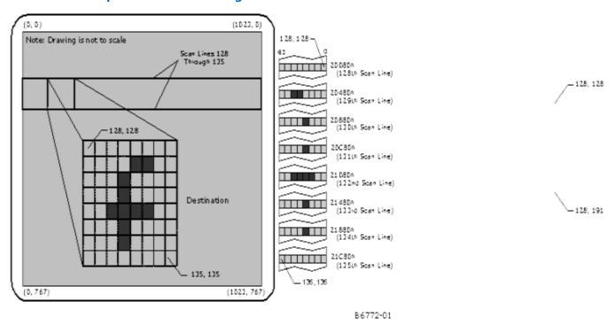
The preceding shows the end result of performing this BLT operation. Only the pixels that form part of the actual letter "f" have been drawn into the 8x8 destination location on the display, leaving the other pixels within the destination with their original gray color.
