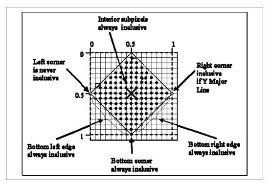
The solid-colored subpixels are considered "interior" to the diamond centered on the pixel sample point. Here the Manhattan distance to the pixel sample point (center) is less than  $\frac{1}{2}$ .
