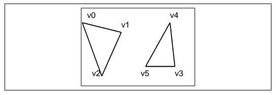
The decomposition process divides the list into a series of basic 3DOBJ\_TRIANGLE objects that are then passed individually and in order to the Object Setup stage. The triangles are generated with the following object vertex order: v0,v1,v2; v3,v4,v5; and so on. The *provokingVertex* of each object is taken from the **Triangle List/Strip Provoking Vertex Select** state variable, as programmed via SF\_STATE.
