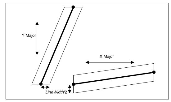
Figure 7-16. Non-Antialiased Line Rasterization
