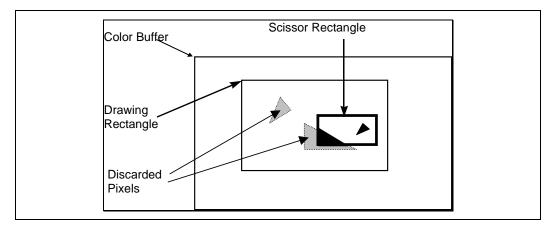
The (DEBUG ONLY) **Fast Scissor Clip Disable** state variable in SF\_STATE controls how scissor clipping is implemented (though this does not affect the rendered image). If ENABLED (i.e., fast clipping is enabled), only those pixels within the scissor rectangle are rasterized. If DISABLED, the entire object will be rasterized, with object pixels falling outside the scissor rectangle being discarded.
