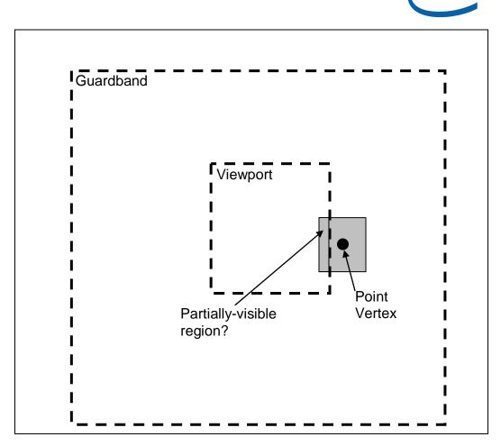
In general, OpenGL dictates that the partially-visible region must not be rendered. In this case the point must be TR against the VPXY (not TA against the GB). To accomplish this, SW could disable the GB when drawing wide points.
