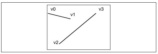
The decomposition process divides the list into a series of basic 3DOBJ\_LINE objects that are then passed individually and in order to the Object Setup stage. The lines are generated with the following object vertex order: v0, v1; v2, v3; and so on. The *provokingVertex* of each object is taken from the **Line List/Strip Provoking Vertex Select** state variable, as programmed via SF\_STATE.
