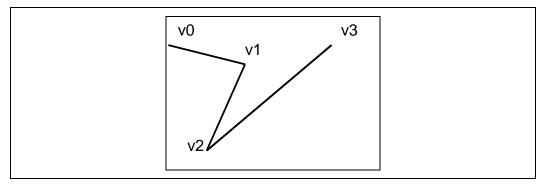
The decomposition process divides the strip into a series of basic 3DOBJ\_LINE objects that are then passed individually and in order to the Object Setup stage. The lines are generated with the following object vertex order: v0,v1; v1,v2; and so on. The *provokingVertex* of each object is taken from the **Line List/Strip Provoking Vertex Select** state variable, as programmed via SF\_STATE.
