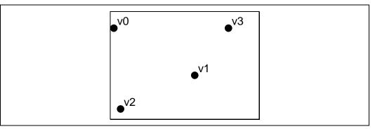
The decomposition process divides the list into a series of basic 3DOBJ\_POINT objects that are then passed individually and in order to the Object Setup subfunction. The *provokingVertex* of each object is, by definition, v[0].
