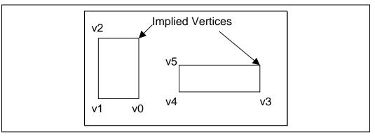
The decomposition of the 3DPRIM\_RECTLIST primitive is identical to the 3DPRIM\_TRILIST decomposition, with the exception of the *objectType* variable.
