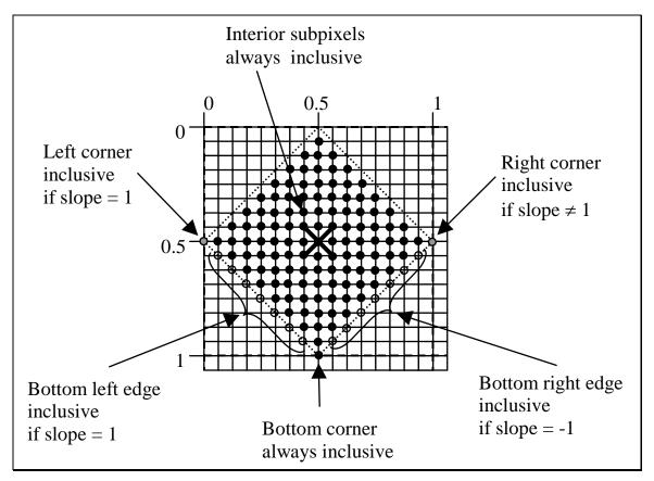
The solid-colored subpixels are considered "interior" to the diamond centered on the pixel sample point. Here the Manhattan distance to the pixel sample point (center) is less than  $\frac{1}{2}$ .
