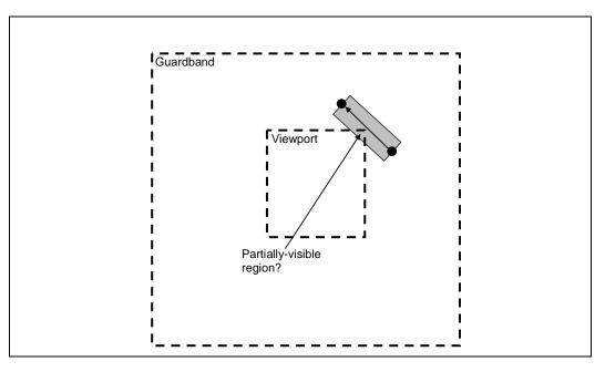
In general, OpenGL dictates that the partially-visible region must not be rendered. In this case the line must be clipped-out against the VPXY (not TA against the GB). To accomplish this, SW could disable the GB when drawing wide lines.
