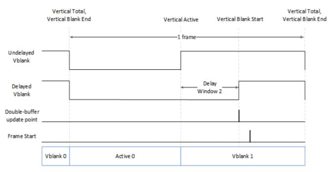
When variable refresh rate is used, the vblank stretches while waiting for the indication to complete this vblank and start the next frame. The stretching happens before window 2.
