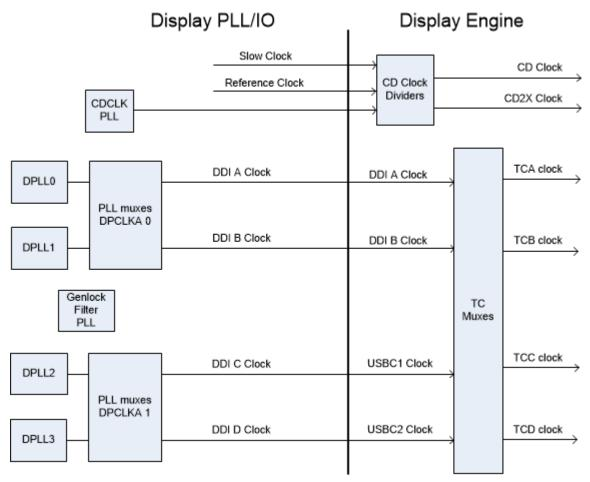
The PLL has two separate PLL to DDI muxes, allowing limited combinations of PLL to DDI mapping. DPLL0 and DPLL1 can be directed to DDIA or DDIB clock. Controlled by DPCLKA0\_CFGCR0. DPLL2 and DPLL3 can be directed to DDIC (USBC1) or DDID (USBC2) clock. Controlled by DPCLKA1\_CFGCR0.
