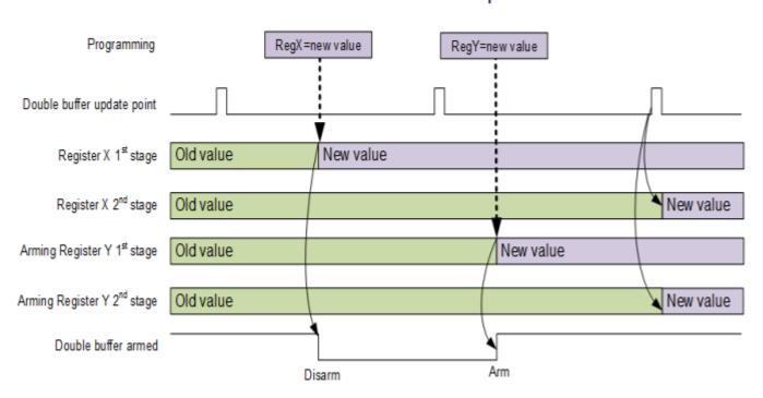
Note: Once armed, by writing to the armed by register, the registers controlled by this arming should not be changed until the double buffer update point is reached. If changed, this will disarm the sequence and will require another write to the armed by register to get it to the armed status again.
