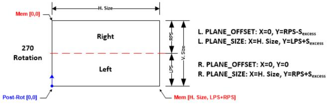
Note that Software should ensure that the horizontal Plane position for the image in the right Pipe is zero (i.e. there should be no positional offset of the image with respect to the seam)
