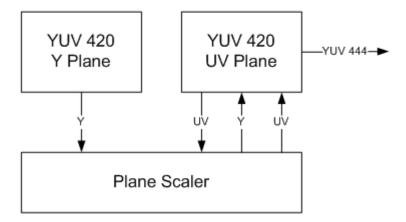
Destination keying, Color correction and Gamma must be programmed in the UV plane. Destination keying, Color correction and Gamma programming in the Y plane gets ignored. The UV plane position is used for blending order determination.
