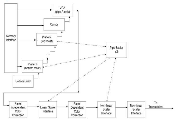
The display pipes contain the planes, blending, color measurement and adjustment, scaling, and dithering.
