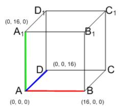
The LUT entries should start at A and end at C<sub>1</sub> following the sequence specified below.
