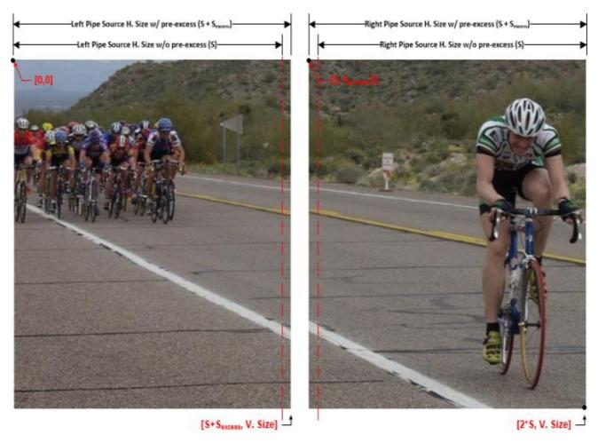
Note that this discussion assumes symmetric horizontal Pipe Source Sizes without the source excess (i.e. S) across both Pipes. This is not a requirement, but it will be left to the reader to extrapolate the equations within this section for asymmetric S terms.
