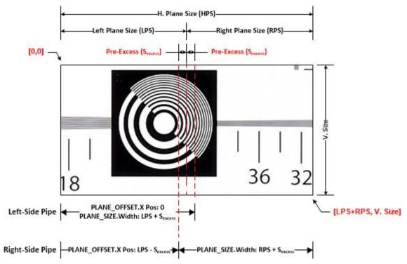
Using the figure above as a reference, to split the image in memory across the two Pipes. Left PLANE\_OFFSET:
