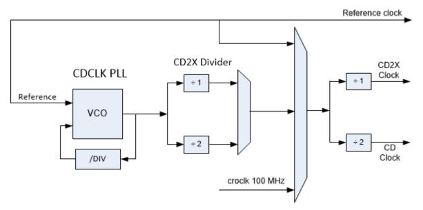
The CDCLK PLL is the main source for CD clock. A programmable divider inside the PLL controls the PLL frequency. The CD2X Divider after the PLL provides additional dividing to create the CD2X clock used by the display engine. The programmable divider value must be set to account for the reference frequency for in the **DSSM** Reference Frequency field.
