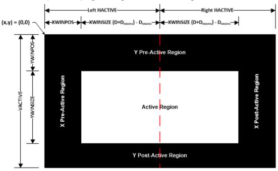
As we can see from the above illustration, the left-side border is applied by the PS\_WIN\_POS programming of the left-side Scaler and the right-side border is applied by the H. Active programming of the right-side transcoder.
