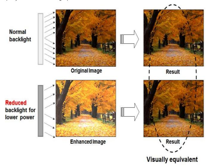
DPST generates statistics (histogram) for each image frame that is sent to the display. These statistics are used to determine if, and by how much, the backlight level can be reduced, saving backlight power. In order to maintain the same image brightness, the image pixel values are increased by an amount related to the backlight level reduction.
