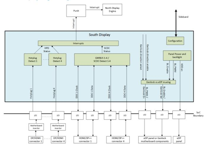
The South Display Engine supports Hot Plug Detection, Panel Power Sequencing, Backlight Modulation, GMbus DDC, and motherboard genlock direction controls.
