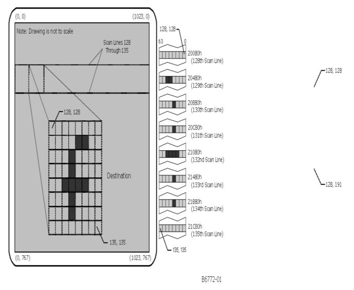
The preceding shows the end result of performing this BLT operation. Only the pixels that form part of the actual letter "f" have been drawn into the 8x8 destination location on the display, leaving the other pixels within the destination with their original gray color.
