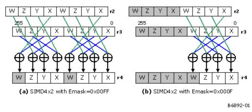
The two source operands only need to be 16-byte aligned, not have to be GRF register aligned. For example, the first source operand could be a 4-element vector (e.g. a constant) stored in doublewords 0-3 in r2, which is shared by the two program flows. The example 3D graphics API Shader instruction can then be translated into the following GEN instruction:
