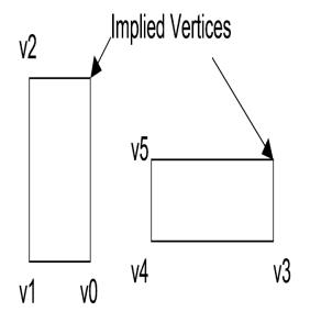
The decomposition of the 3DPRIM\_RECTLIST primitive is identical to the 3DPRIM\_TRILIST decomposition, with the exception of the *objectType* variable.
