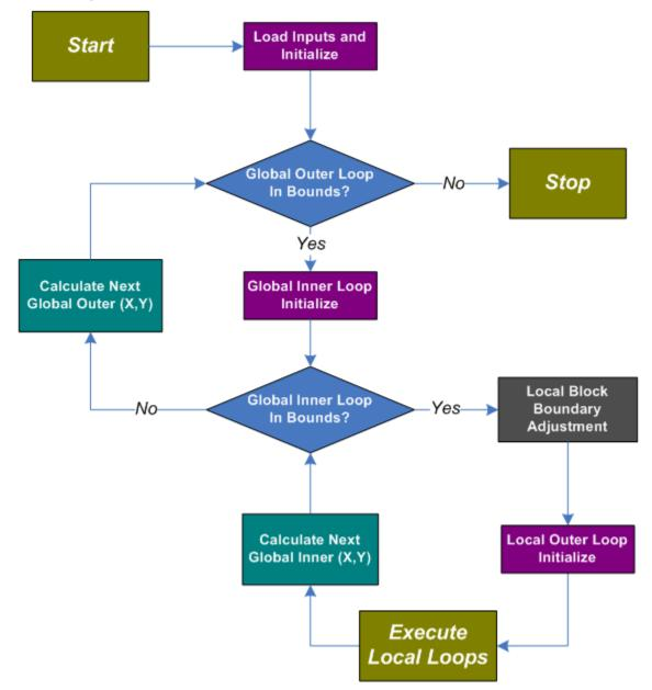
Take note of the grey box "Local Block Boundary Adjustment". This logic is necessary to adjust the local block size when the distance between the current global position to the edge of the image is less than the local resolution. Additionally, the local starting positions might be modified here as well if the defined starting position is larger than the new local block size.
