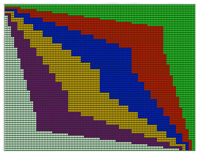
Each color indicates a separate segment which is dispatched to a different subslice.
