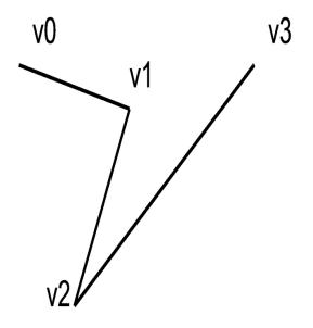
The decomposition process divides the strip into a series of basic 3DOBJ\_LINE objects that are then passed individually and in order to the Object Setup stage. The lines are generated with the following object vertex order: v0,v1; v1,v2; and so on. The *provokingVertex* of each object is taken from the **Line List/Strip Provoking Vertex Select** state variable, as programmed via SF\_STATE.
