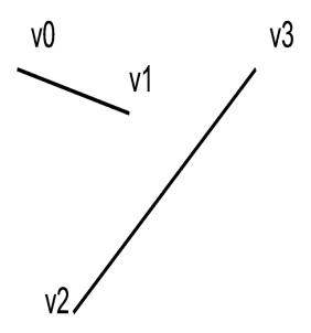
The decomposition process divides the list into a series of basic 3DOBJ\_LINE objects that are then passed individually and in order to the Object Setup stage. The lines are generated with the following object vertex order: v0, v1; v2, v3; and so on. The *provokingVertex* of each object is taken from the **Line List/Strip Provoking Vertex Select** state variable, as programmed via SF\_STATE.
