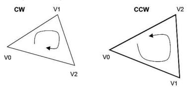
The **Front Winding** state variable in SF\_STATE controls whether CW or CCW triangles are considered as having a "front-facing" orientation (at which point non-front-facing triangles are considered "back-
