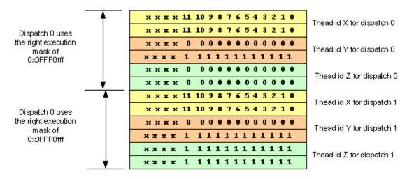
The width and height counter would have a maximum of 1, and the depth counter would have a maximum of 2. The two dispatches would use the AND of the two masks, but since the bottom mask is F it would be the same as just the right mask.
