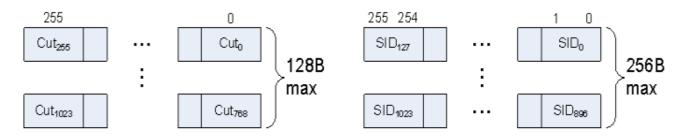
Following the optional header is a variable number of 16B or 32B-aligned/granular vertices:
