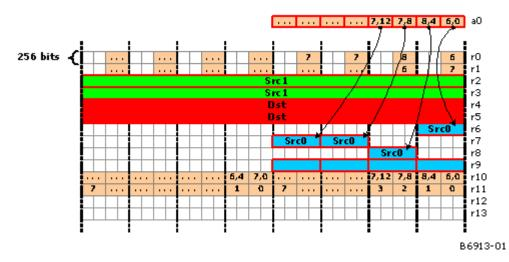
Without vector immediate support, such translation has to either use a long sequence of scalar instructions which is very inefficient or use a constant load which requires additional constant to be managed in memory.
