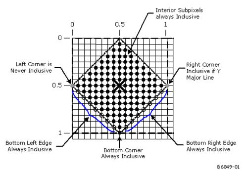
The solid-colored subpixels are considered "interior" to the diamond centered on the pixel sample point. Here the Manhattan distance to the pixel sample point (center) is less than  $\frac{1}{2}$ .
