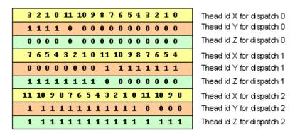
In this case the thread counter width would be programmed with a maximum value of 3 (since all the execution masks are all F, it doesn't matter how the thread counters are programmed as long as they count to 3 before finishing the thread group).
