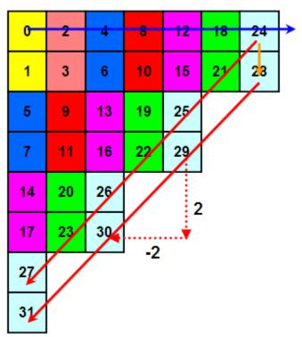
The outer loop unit step vector would be [1, 0] and the inner loop unit step vector would be [-2, 2]. A third loop is necessary to repeat the inner loop, only shifted down a unit before restarting. Thus, a middle loop with a unit step vector of [0,1] would achieve this MBAFF pattern. Additionally, the number of "extra steps" taken by the middle loop would be 1 in this case.
