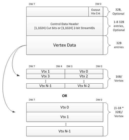
The following diagram illustrates the possible layouts of a GS URB Entry:
