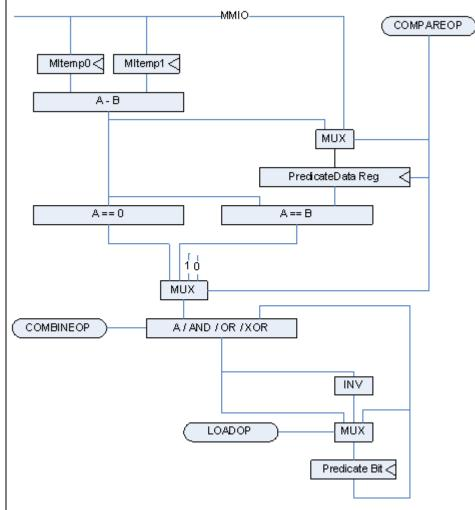
MI\_LOAD\_REGISTER\_MEM commands can be used to load the MItemp0, MItemp1, and PredicateData registers prior to MI\_PREDICATE. To ensure the memory sources of the MI\_LOAD\_REGISTER\_MEM commands are coherent with previous 3D\_PIPECONTROL store-DWord operations, software can use the new **Pipe Control Flush Enable** bit in the PIPE\_CONTROL command.
