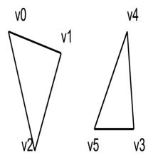
The decomposition process divides the list into a series of basic 3DOBJ\_TRIANGLE objects that are then passed individually and in order to the Object Setup stage. The triangles are generated with the following object vertex order: v0,v1,v2; v3,v4,v5; and so on. The *provokingVertex* of each object is taken from the **Triangle List/Strip Provoking Vertex Select** state variable, as programmed via SF\_STATE.
