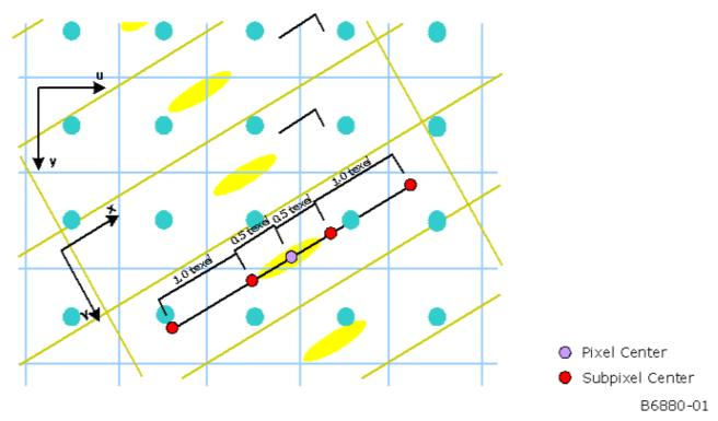
Each subpixel samples a bilinear 2x2 around it just as if it was a single pixel. The result of each subpixel is then blended together using equal weights on all interior subpixels (not including the two endpoint subpixels). The endpoint subpixels have lesser weight, the value of which depends on how close the "ratio" is to the number of "ways". This is done to ensure continuous behavior in animation.
