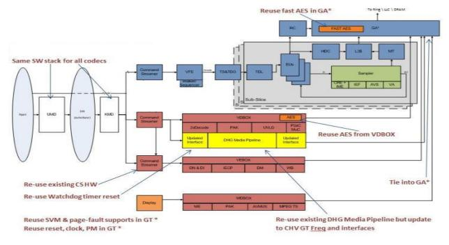
**CHV, BSW GT Media Pipelines:** This solution maximizes re-use of existing assets while providing legacy codec coverage.
