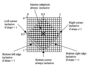
The solid-colored subpixels are considered "interior" to the diamond centered on the pixel sample point. Here the Manhattan distance to the pixel sample point (center) is less than <sup>1</sup>/<sub>2</sub>.
