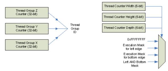
The X/Y/Z counters for the thread group will have an initial and maximum value. The thread group ID sent with each dispatch consists of these 3 numbers. These counters are 32 bits since the spec does not limit the size of the thread ID.
