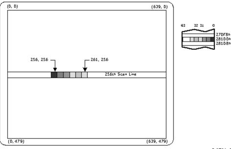
**Representation of On-Screen Single 6-Pixel Line in the Frame Buffer**
