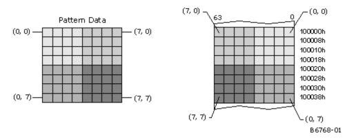
As shown in figure above, the pattern data occupies 64 bytes starting at address 100000h. As always, the pattern data represents an 8x8 array of pixels.
