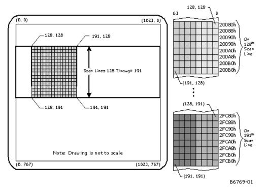
The figure above shows the end result of performing this BLT operation. The 8x8 pattern has been repeatedly copied ("tiled") into the entire 64x64 area at the destination.
