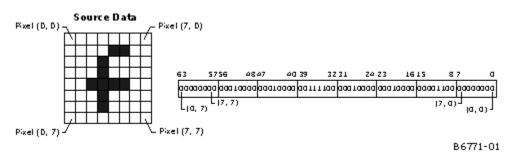
The figure above shows both the 8x8 pattern making up the letter "f" and how it is represented somewhere in the host's system memory — the actual address in system memory is not important. The letter "f" is represented in system memory by a block of monochrome graphics data that occupies 8 bytes. Each byte carries the 8 bits needed to represent the 8 pixels in each scan line's worth of this graphics data. This type of pattern is often used to store character fonts in system memory.
