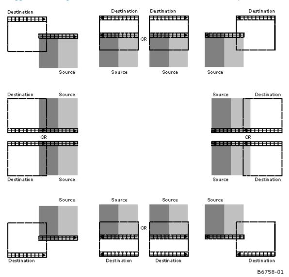
The figure above shows the recommended lines and pixels to be used as starting points in each of 8 possible ways in which the source and destination locations may overlap. In general, the starting point should be within the area in which the source and destination overlap.
