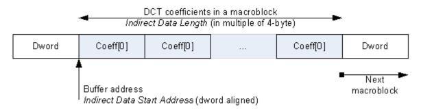
Each non-zero coefficient in the indirect data buffer is contained in a doubleword-size data structure consisting of the coefficient index, end of block (EOB) flag and the fixed-point coefficient value in 2's compliment form. As shown in *Common Indirect IT-COEFF Data Structure*, *index* is the row major 'raster' index of the coefficient **within a transform block** (*please note that it is not converted to 8x8 block basis*). A coefficient is a 16-bit value in 2's complement.
