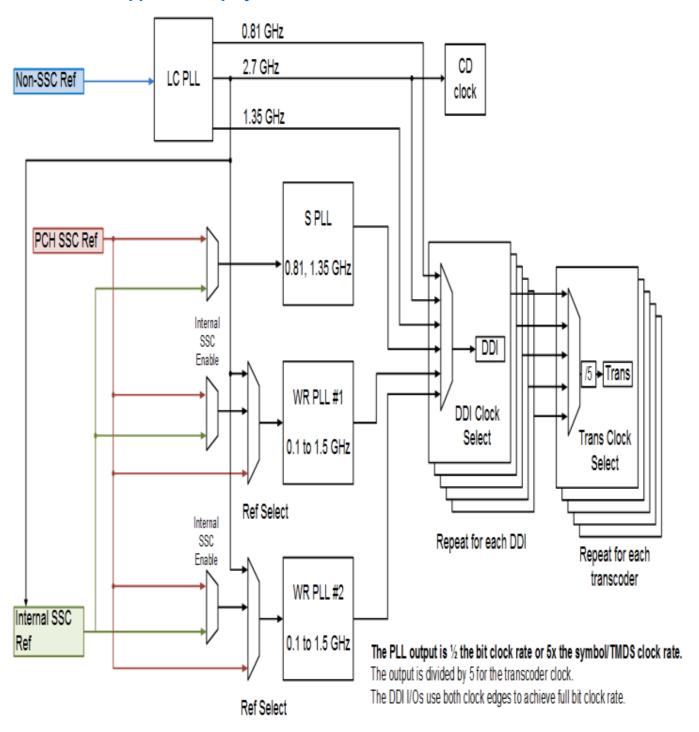
The display engine clocking structure has multiple reference clocks, PLLs, and clocks. The general flow is from reference to PLL to DDI (port) clock to transcoder clock.
