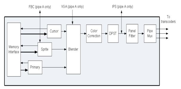
The display pipes contain the planes, blending, color correction, DPST, panel fitting, dithering, and clipping.
