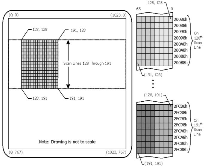
The figure above shows the end result of performing this BLT operation. The 8x8 pattern has been repeatedly copied ("tiled") into the entire 64x64 area at the destination.
