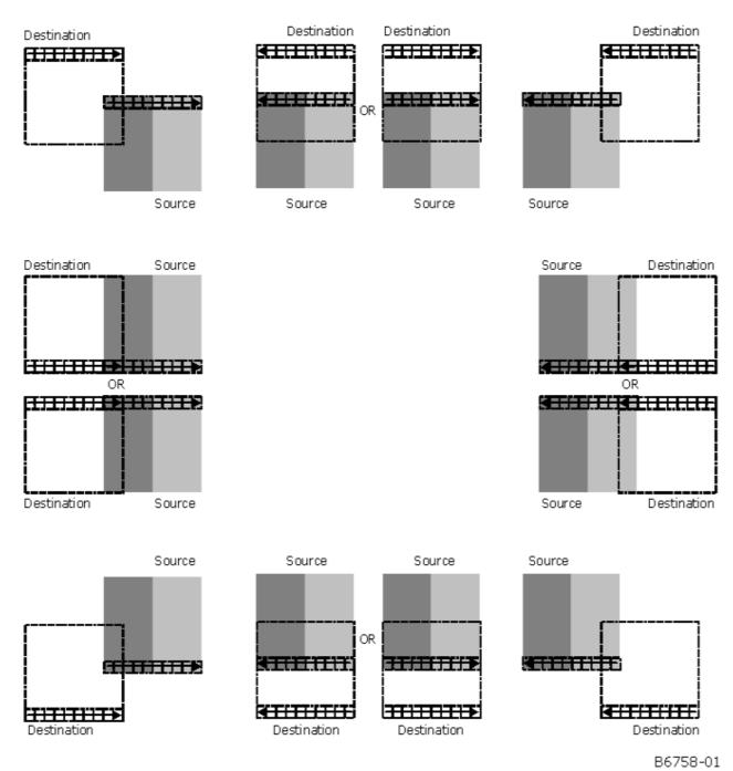
The figure above shows the recommended lines and pixels to be used as starting points in each of 8 possible ways in which the source and destination locations may overlap. In general, the starting point should be within the area in which the source and destination overlap.
