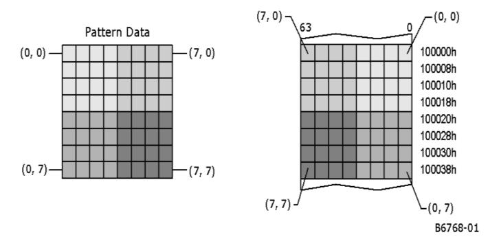
As shown in figure above, the pattern data occupies 64 bytes starting at address 100000h. As always, the pattern data represents an 8x8 array of pixels.
