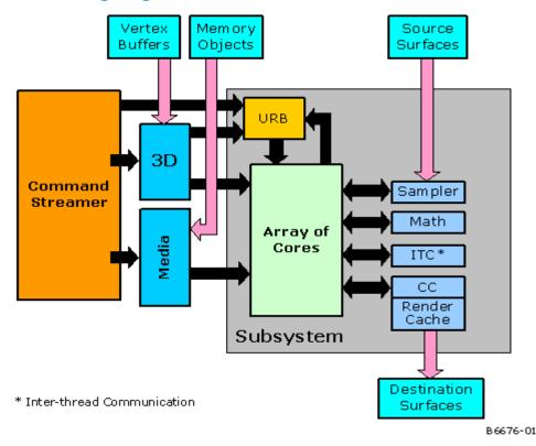
The subsystem consists of an array of *execution units* (*EUs* along with a set of *shared functions* outside the EUs that the EUs leverage for I/O and for complex computations. Programmers access the subsystem via the 3D or Media pipelines.
